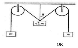
Determine the tensions  $T_1$  and  $T_2$  in the strings shown in figure.
